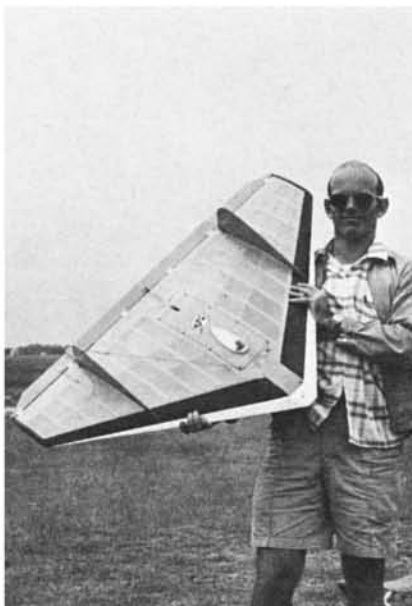
Skip Schow flew his Midwest Delta Hustler, after the contest. Ship is modified to be a slope soarer, engine removed and nose filled in.
